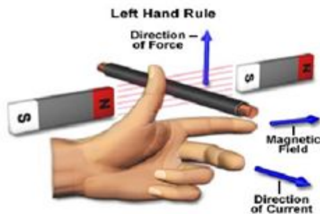
Fig. 5.2.2 Fleming Left Hand Rule
